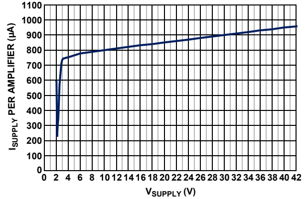
FIGURE 26. SUPPLY CURRENT vs SUPPLY VOLTAGE
